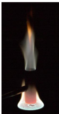
Picture of pre-mixed flame and chimney for material flame synthesis of nanomaterials.
